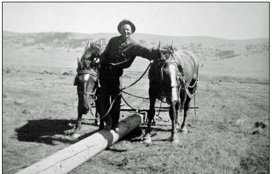
Figure 5. These images provide two views of a plunger used with a beaverslide stacker, which was used to create large 20' X 24' X 20' stacks in the ranch's meadows. Rather than pulling, the team pushed the device which moved the hay onto the stack. The plunger was 38 feet long and made from the trunk of a lodgepole pine. SOURCE: Carole Settele Anderson photographic collection, undated.
