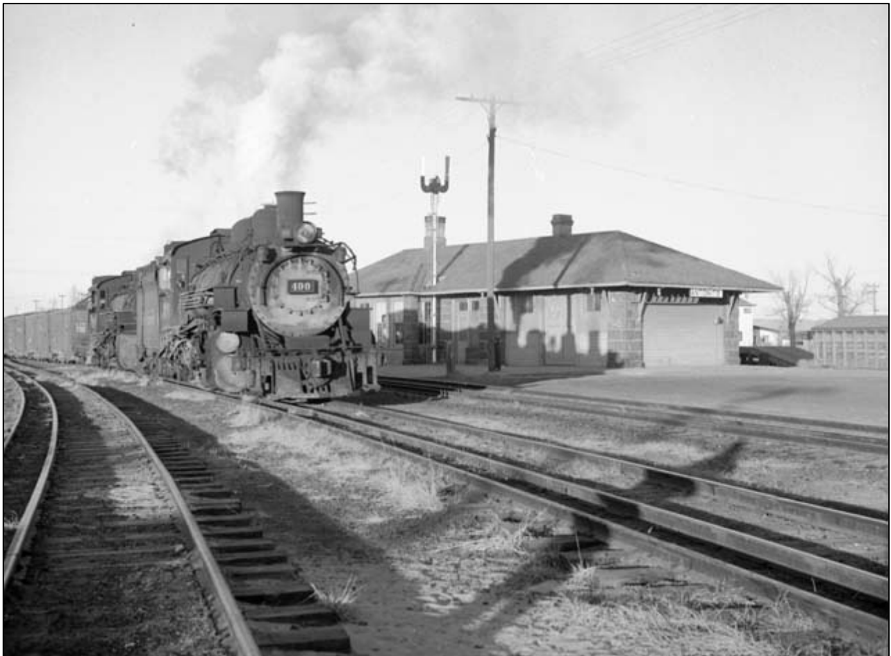
Figure 2. A west-bound freight train passes the west side of the Antonito Depot on January 29, 1958. The three sets of tracks contain three rails each to accommodate both narrow gauge and standard gauge cars. Photographer: Robert W. Richardson. Source: Western History / Genealogy Department, Denver Public Library.
