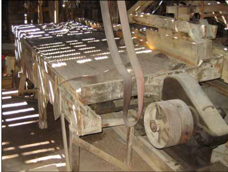
Figure E 96: Following its introduction around 1898, the vibrating table was one of the most popular and effective concentration appliances throughout the Rocky Mountain west. An eccentric cam under the guard at right imparted a vibrating motion to the tabletop, and the vigorous action caused heavy metalliferous material to settle against the riffles. Water currents washed the light waste off. Source: Carol Beam, Boulder County Parks and Open Space.
